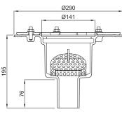
Model with vertical outlet socket DN 50
