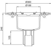
Model with vertical outlet socket DN 80
